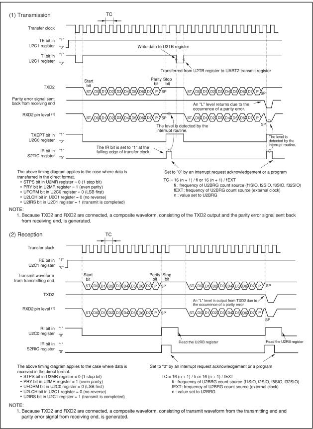
Figure 14.32 Transmit and Receive Timing in SIM Mode
